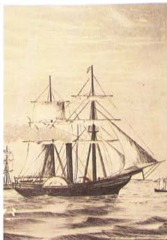
Sophia Jane is the first 'auxiliary steamer'—a ship powered by both sail and steam—to reach Australia. Undated etching by T.R. Amies.
